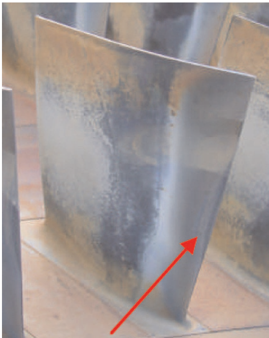
Fig. 19 Water stain on the suction side of blade row 8 of a 60 Hz unit
