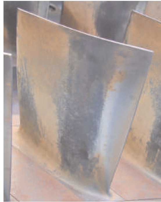
Fig. 20 Absence of water stains on blade row 9 of a 60 Hz unit
